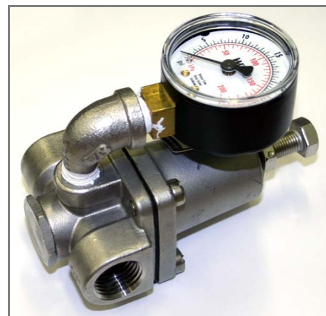
Figure 2: Pressure reduction valve (Shown uninstalled)
